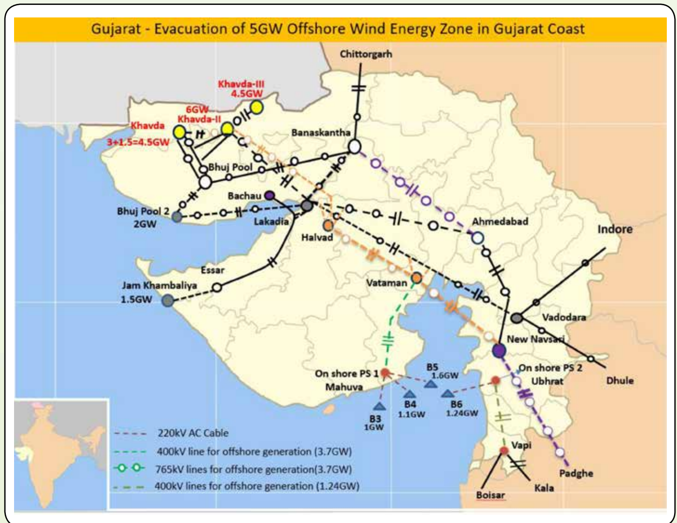
Fig. 3: Transmission system for off-shore wind potential zones in Gujarat
